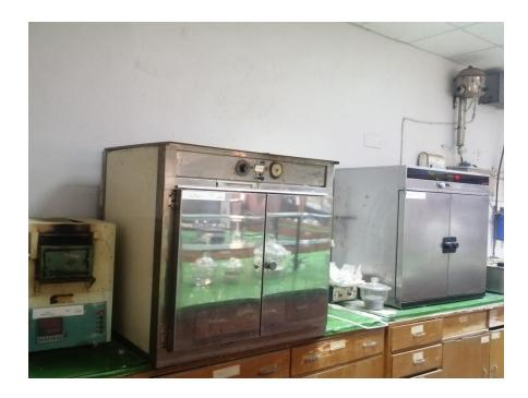
• Muffle furnace for calculating the percentage of organic matter in samples and for calculating the percentage of loss on ignition at temperatures up to 1200°C.
